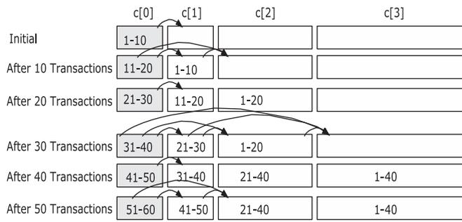
Fig. 10. Value added shifting (batch size  $b = 10$ ). Gray boxes denote windows processing new stream values.
