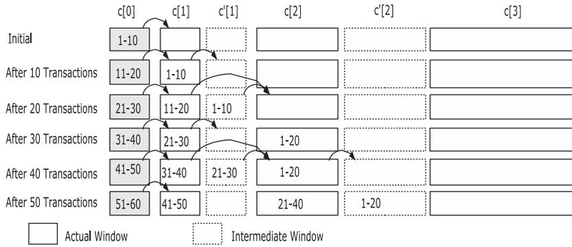
Fig. 6. Shifting with intermediate windows (batch size  $b = 10$ ). Gray boxes denote windows processing new stream values.
