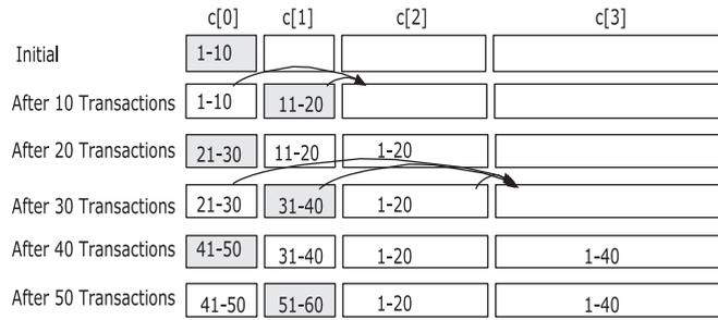
Fig. 8. Shifting without intermediate windows (batch size  $b = 10$ ). Gray boxes denote windows processing new stream values.
