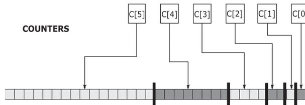
Fig. 4. Tilted-time windows (new items are inserted in the rightmost counter).
