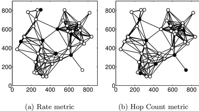
**Fig. 4.** Optimal placement of core nodes (the black circles) in a random topology with  $N = 40$  nodes. Two different cost metrics are compared, namely the hop count and the overall transmission time (rate metric).
