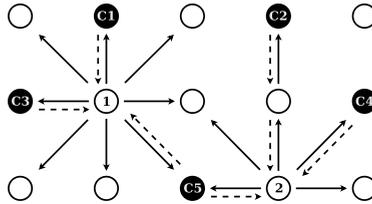
**Fig. 1.** Distributed security architecture: a (5,3) threshold scheme is adopted in this example WMN, where black and white circles represent, respectively, core and generic nodes. Solid lines represent requests, while dashed lines represent core node responses.
