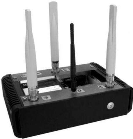
Figure 7: Multi-radio MobiMESH router.
