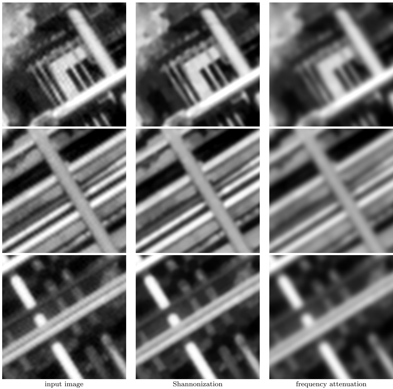
Fig. 13 Details of Fig. 12 with Shannon resampling. Different parts of the three images of the first row of Fig. 12 are shown after Shannon interpolation. As expected, the output of the “Image Shannonizer” (middle) is well interpolable, contrary to the input image (left) on which oscillations appear. A simple frequency attenuation (right) is not efficient, since it introduces a large amount of undesired blur.
