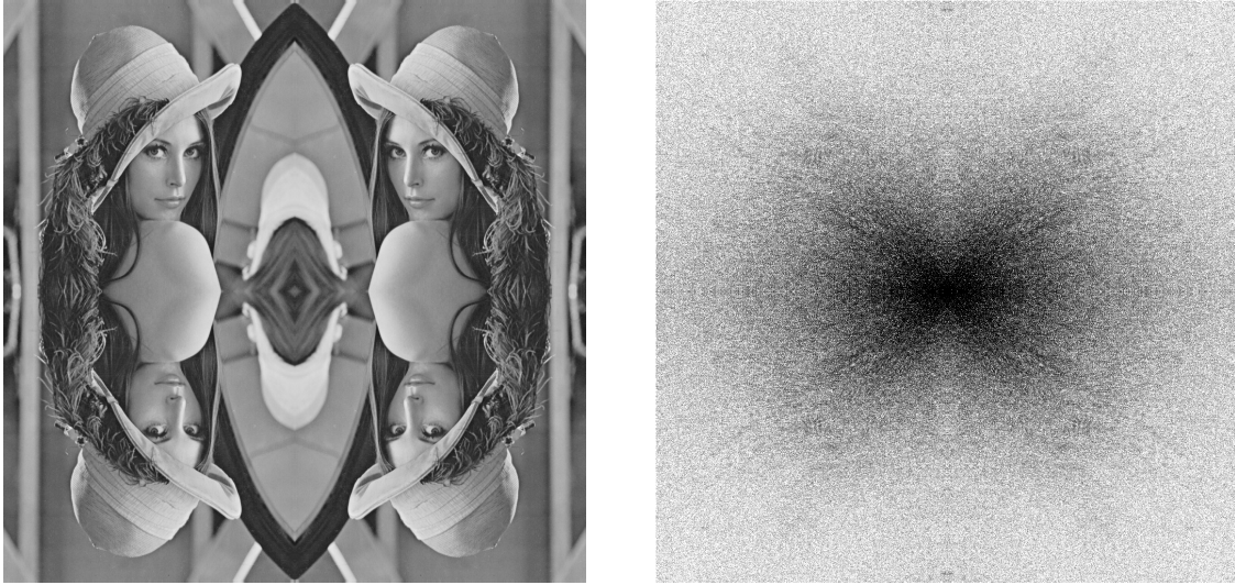
Figure 2: Symmetrization of the Lena image (left) and its corresponding Discrete Fourier Transform (modulus in log scale, right). Compared to Figure 1, the cross structure has disappeared in the Fourier domain, but the price to pay is a loss of information (orientation, phase component) due to the fact that the DFT of a symmetric image is constrained to be a symmetric real-valued function.
