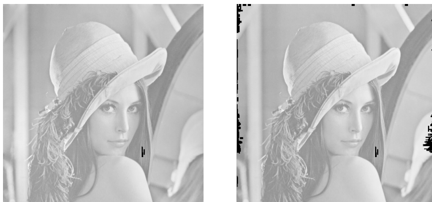
Figure 8: Effect of the periodic plus smooth decomposition on ringing detection. The classical Lena image is submitted to the Shannon-compliance test described in [5], which consists in a Shannon (1/2, 0) translation followed by an a-contrario horizontal ringing detection process (with an expected number of false alarms equal to 0.01). When the periodic component is analyzed (left), ringing detection (marked in black) only occurs in a textured zone (the hair) where horizontally oscillating pattern are expected, which supports the idea that Lena image has been sampled in accordance with Shannon Theorem. When the original image is used directly (right), a lot of spurious detections arise on the frame border.
